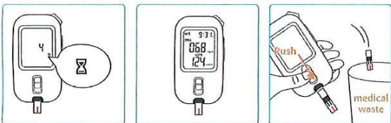
The countdown indicates testing in progress. The results appear on the screen at the end of the countdown. Remove the strip.
